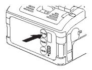
2. Push the black release lever (1) down and toward the front of the printer to open the cover
